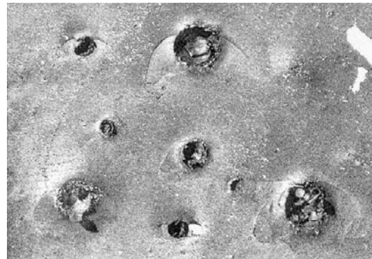
Fig. 2 Crack propagation from carbon black. Detailed section plot of cracked specimen by Gent (Magn. 13.)
